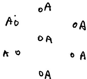
The spacing between nearest neighbor points of the Bravais lattice is  $\sqrt{3}a$ , where  $a$  is the lattice spacing of the honeycomb lattice.
